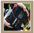
The built in charger point on the handlebar allows the charger to be connected without removing the rear cover. For off machine charging, the battery is simply removed.
