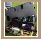
Removable cover provides protection and allows easy access to the electrics, pump and battery. The cover is manufactured from precision moulded MDPE.
